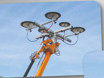
The Smartlift has hydraulic movements in all directions
