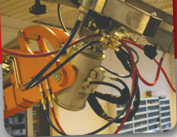
The multifunktiyonel, hydraulic rotary head
