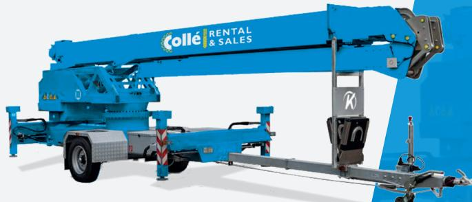
The K300E demonstrates that power and durability can be perfectly combined. Thanks to the 22 kW lithium iron phosphate battery, this crane operates fully electrically. It can drive and lift without emissions, operating quietly, cleanly, and powerfully.
