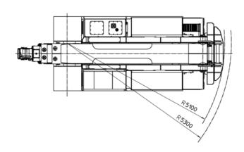
FRAME: JMG designed and manufactured, box type, torsion resistant design of high strength structural steel.
