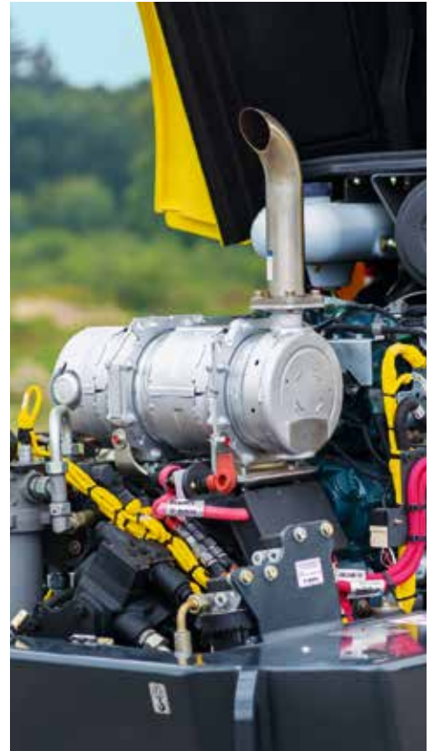
All cables are protected against damage.
