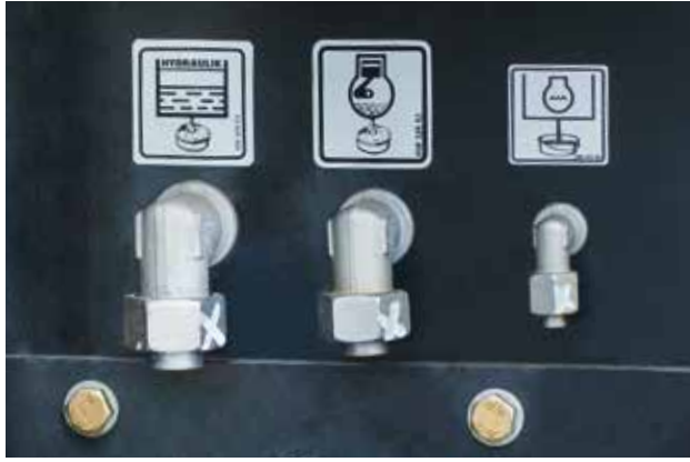
Smart: operating materials can be drained externally.
