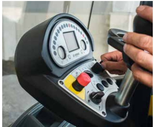
Operating controls: logical arrangement and self-explanatory.
