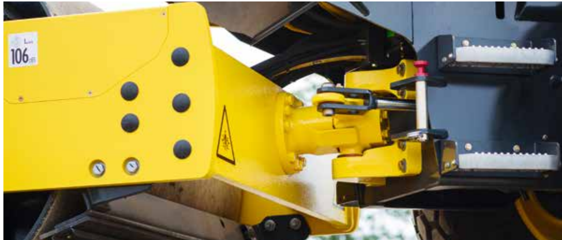
Clean-cut: The articulated joint is maintenance-free; the machine needs no manual greasing whatsoever.
