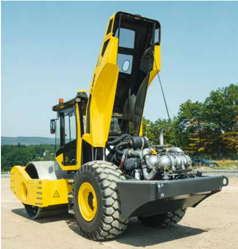
Handy, large, hinged hood: all service points are easily accessible.
