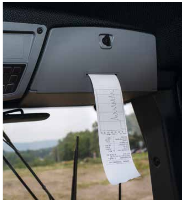
Integrated printer: for documentation of compaction results.
